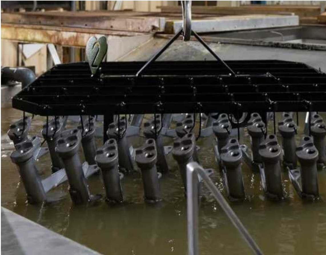
Surface treatment of hollow and complicated shapes, as well as small, large-numbered workpieces
